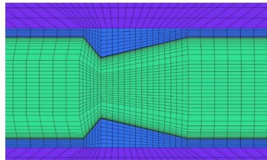
**Figure 5.** Axial section diagram of CD-PTR mesh.
