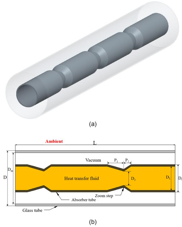
**Figure 3.** 3D view and axial section schematic of CD-PTR studied in this paper.
