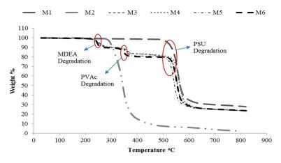
Figure 6. Effect of TGA on enhanced polymeric blend membranes with various composition of PVAc in PSU with MDEA amine
