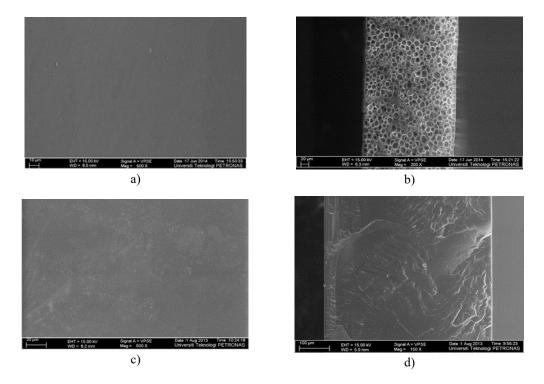
**Figure 3.** a) Top view (500 X), b) cross section view (200 X) of PSU based membrane and c) top view (500 X), (d) cross section view (200 X) of PVAc based membrane
