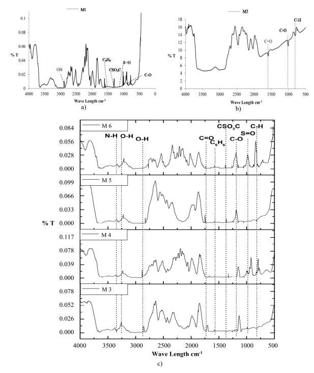
**Figure 7.** FTIR of spectral analysis a) based PSU membrane, b) Based PVAc membrane, c) Comparative FTIR spectra of the polymeric blend membranes with MDEA
