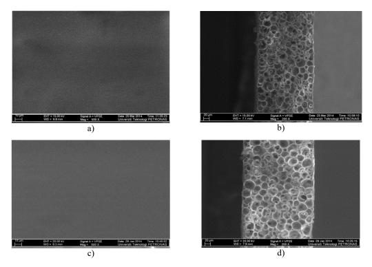
Figure 4. a) Top view (500 X), b) cross section view (200 X) of blend membrane PSU 95% / PVAc 5% / MDEA and c) top view (500 X), d) cross section view (200 X) of blend membrane PSU 90% / PVAc 10% / MDEA
