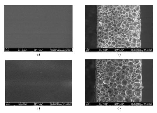
Figure 5. a) Top view (500 X), b) cross section view (200 X) of blend membrane PSU 85% / PVAc 15% / MDEA and c) top view (500 X), d) cross section view (200 X) of blend membrane PSU 80% / PVAc 20% / MDEA
