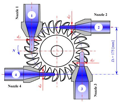
Figure 4. Configuration of nozzles in hydro Turgo turbine
