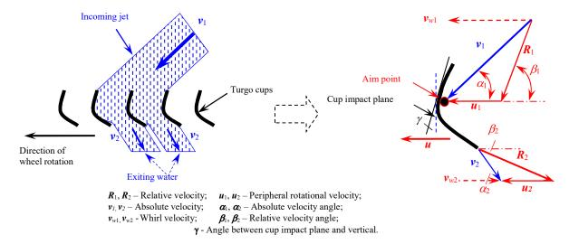
Figure 3. Velocity triangles of hydro Turgo turbine
