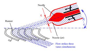
Figure 1. Direction of water flow for hydro Turgo turbine
