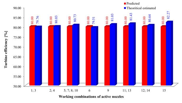
**Figure 9**. Predicted and estimated values of turbine efficiency as a function of the working combinations of active nozzles of the micro hydro Turgo turbine
