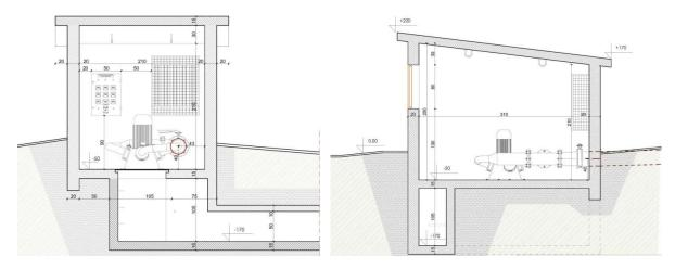
Figure 6. Top and front view of the micro hydro Turgo turbine house
