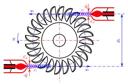
Figure 2. Design parameters of the hydro Turgo runner
