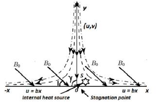
Figure 1. Schematic diagram for orthogonal flow
