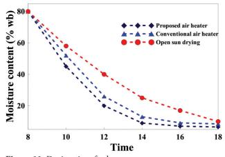
Figure 11. Drying time for banana.
