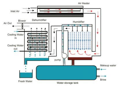
Figure 2. Proposed humidification – dehumidification desalination system.
