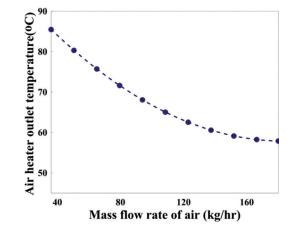
Figure 6. Effect of air mass flow rate on outlet temperature of air.
