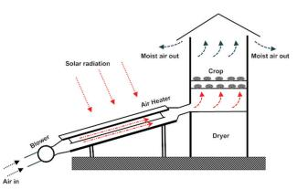
Figure 3. Proposed indirect solar drying system.
