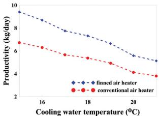
Figure 9. Cooling water temperature vs productivity.
